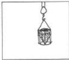
Growing medium raised to the roof in a bucket.
